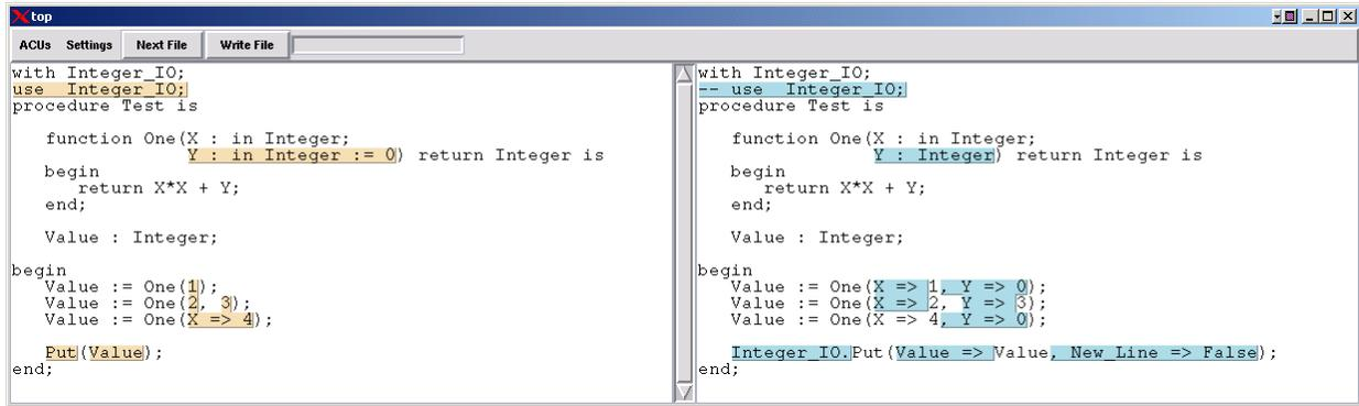
**Figure 1.** The prototype tool in action. The pane on the left shows the original program. Parts of the program that must be changed are highlighted. The pane on the right shows the program after the changes have been applied. Any single transformation can be undone by clicking on it in the right pane.
