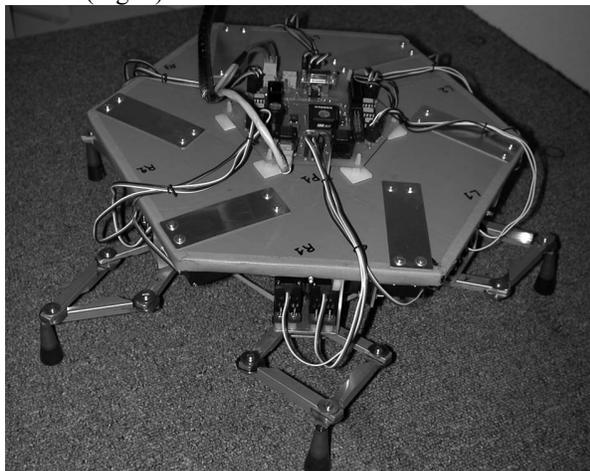
**Figure 1. Bunny, the omnidirectional robot**
