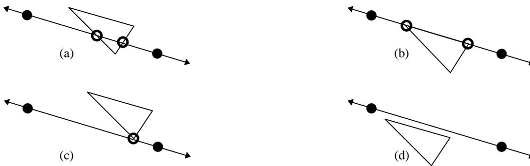
**Figure 3.** The four possible outcomes of the intersection between a facet and the line segment formed from the line of intersection: (a) Intersection at two points; (b) Intersection along an edge; (c) Intersection at a vertex; (d) No intersection. The line segments used in Step 5 are shown with open circles. In case (c), we use a point instead of a line segment in Step 5.
